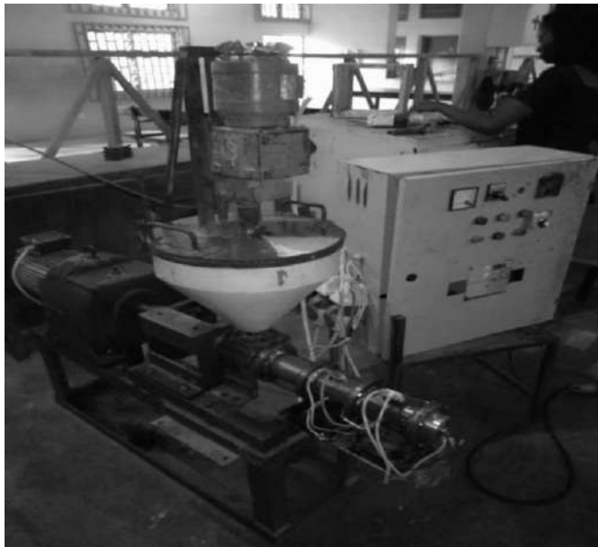
Figure 20: The Laboratory extruder developed
