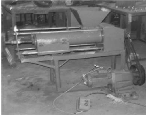
Figure 17: The Developed Oil Palm Screw Press
