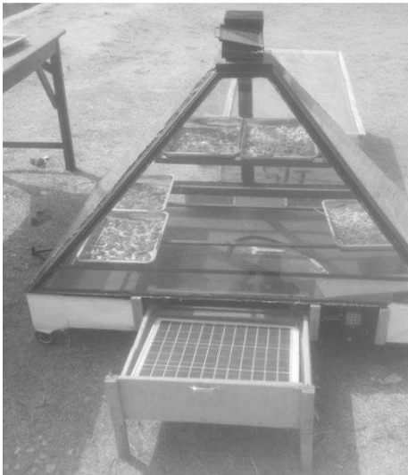
Figure 28: Mobile photovoltaic forced air convection dryer
