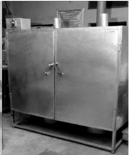
Figure 29: Laboratory scale hot air dryer
