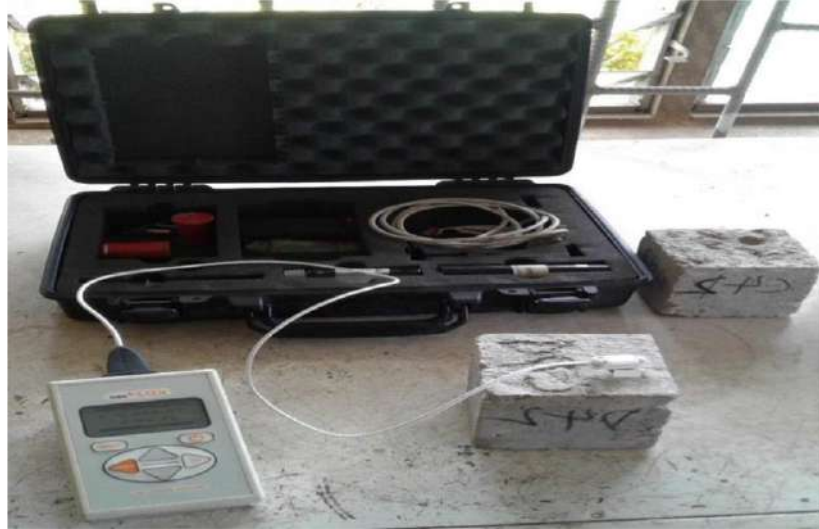
Figure 16: Experimental set-up for determination of thermal properties using KD2 Pro-thermal properties analyzer
