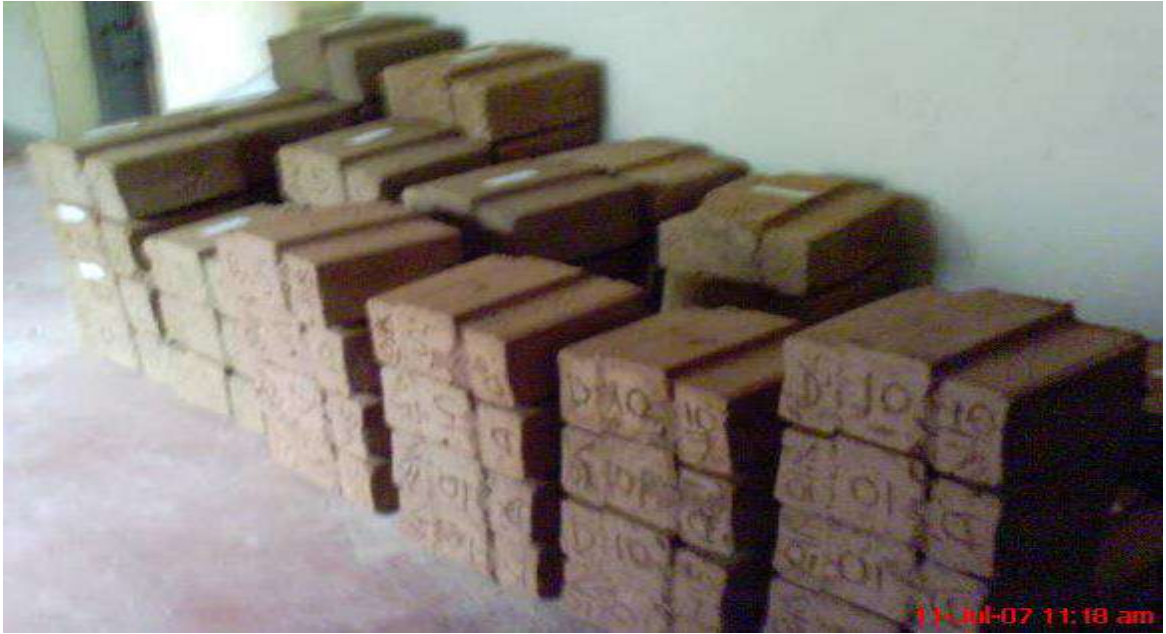
Figure 5: Stacking of Lateritic Interlocking Blocks
