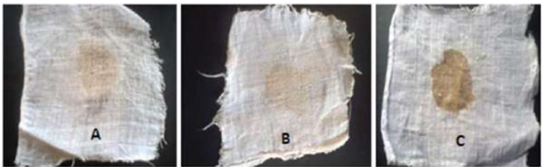
Figure 22: Destaining of blood-stained cloth by crude keratinases. Note: Destaining of blood by the wild-type strain after 3 h of incubation (A), by the mutant strain after 2 h of incubation (B) vs. a control (C) incubated in water
