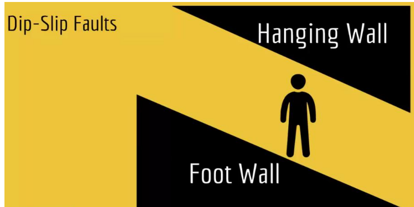
Figure 7: Representation of dip-slip faults
