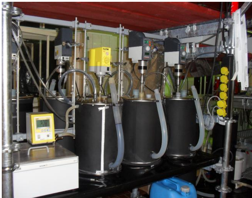
Plate 4: Set up of Continuously Stirred Tank Reactor (CSTR)
