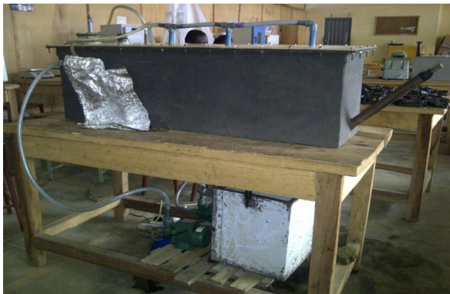
Plate 5: The Plug Flow Reactor in Use Source: Adebayo et al. (2014c)
